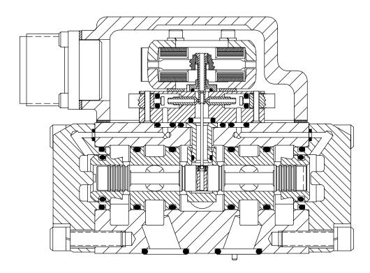
Eaton Vickers® SM4-20 servo valves can provide system closed loop control with exact positional accuracy, repeatable velocity profiles, and predictable force or torque regulation.
