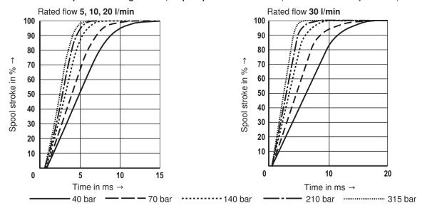
Frequency response with pressure rating 315 bar, stroke frequency without flow (measured with safety barrier 1)
