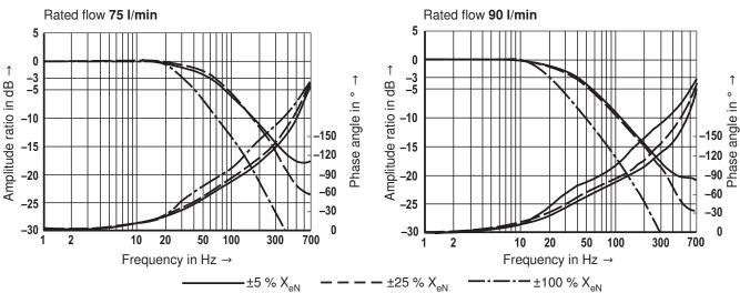
Dependency of the frequency f at -90 ° on the operating pressure p and the inlet amplitude (measured with safety barrier  $^{1)}$ )
