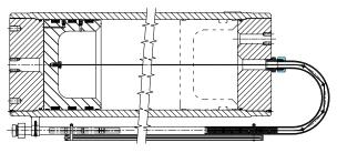
With the magnetic flags indicator, the position of a piston can be determined by the colour (white/red) of a set magnetic flags which turn when the piston moves and which are visible externally.
