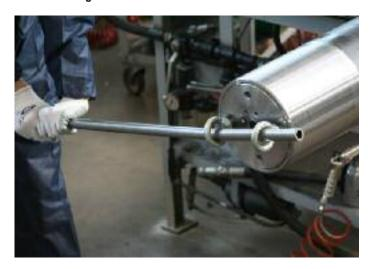
Gas pressure should always be discharged before the disassembly of an accumulator AP. Those accumulators have the oil and gas end caps threaded into the pipe. Always remove the gas cap first – identifiable by the gas valve or by a gas bottle connection.
