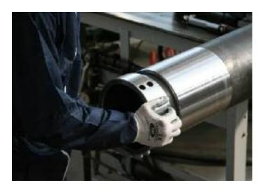
Coat all internal parts with clean hydraulic fluid before reassembly. In order to protect the piston seals and for ease assembly purposes, the use of a loading sleeve is recommended – details of a suitable loading sleeve can be provided by Epe. To minimize the risk of damage to the piston and seals, it is recommended that the replacement piston assembly should be installed with the accumulator pipe positioned vertically.
