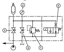
**Note:** When using hydro-pneumatic accumulators for stored hazardous energy, HYDAC recommends the use of its Safety and Shut-off Block (SAF) with solenoid operated bleed valve.
