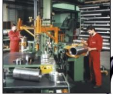
Assembly of piston accumulators
